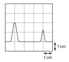
The pulse takes  $6.3\,\mu s$  to travel from the transmitter to the reflector.
